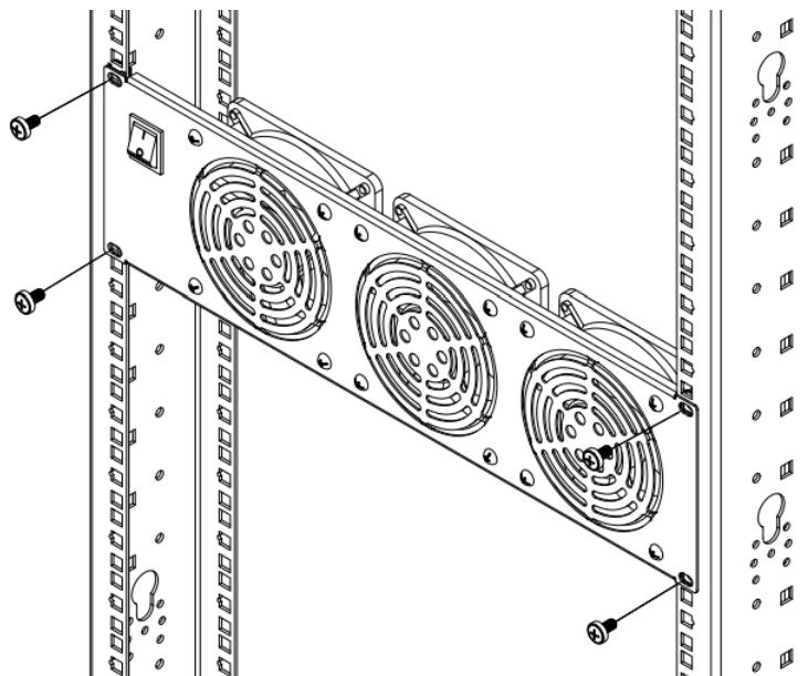
**1** Locate the numbered square openings in the mounting rails where you plan to install your equipment. You will install cage nuts (included) into the square openings to provide an attachment point for the mounting screws (included).
